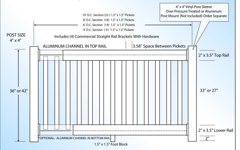
ALL RAILING SECTIONS INCLUDE FOOT BLOCK ON BOTTOM RAIL TO MEET IBC / IRC INTERNATIONAL BUILDING CODE AND RESIDENTIAL CODE NOTE: 10' WIDE SECTIONS INCLUDE TWO FOOT BLOCKS EVENLY SPACED NOTE: \*OPTIONAL ALUMINUM CHANNEL CAN BE ADDED INTO BOTTOM RAIL - CONTACT US FOR PRICING
