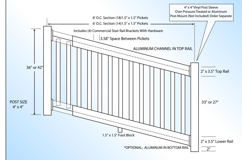
ALL RAILING SECTIONS INCLUDE FOOT BLOCK ON BOTTOM RAIL TO MEET IBC / IRC INTERNATIONAL BUILDING CODE AND RESIDENTIAL CODE NOTE: \*OPTIONAL ALUMINUM CHANNEL CAN BE ADDED INTO BOTTOM RAIL - CONTACT US FOR PRICING
