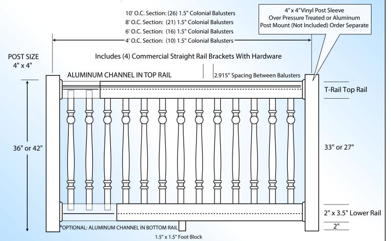
ALL RAILING SECTIONS INCLUDE FOOT BLOCK ON BOTTOM RAIL TO MEET IBC / IRC INTERNATIONAL BUILDING CODE AND RESIDENTIAL CODE NOTE: 10' WIDE SECTIONS INCLUDE TWO FOOT BLOCKS EVENLY SPACED
