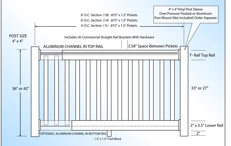
ALL RAILING SECTIONS INCLUDE FOOT BLOCK ON BOTTOM RAIL TO MEET IBC / IRC INTERNATIONAL BUILDING CODE AND RESIDENTIAL CODE NOTE: \*OPTIONAL ALUMINUM CHANNEL CAN BE ADDED INTO BOTTOM RAIL - CONTACT US FOR PRICING
