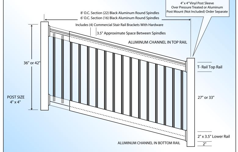
ALUMINUM CHANNEL IN BOTH TOP AND BOTTOM HORIZONTAL RAILS FOR COMMERCIAL STRENGTH. ALL RAILING SECTIONS MEET IBC / IRC INTERNATIONAL BUILDING CODE AND RESIDENTIAL CODE:
