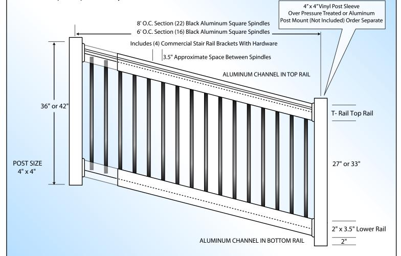
ALUMINUM CHANNEL IN BOTH TOP AND BOTTOM HORIZONTAL RAILS FOR COMMERCIAL STRENGTH.
